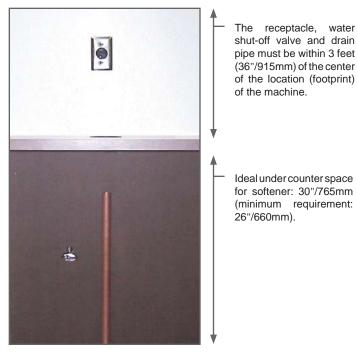
Notes: Access hole is only required if any of the utility hook-ups are located under the counter.
