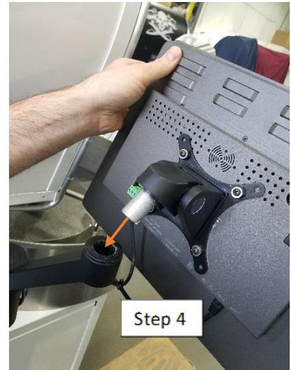
5. Using the screwdriver, re-install the mounting disc in the post of the monitor post and fasten the screw.
