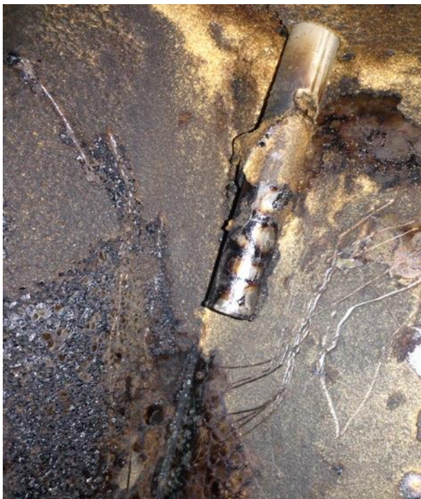
Example of a dirty sensor tube.
