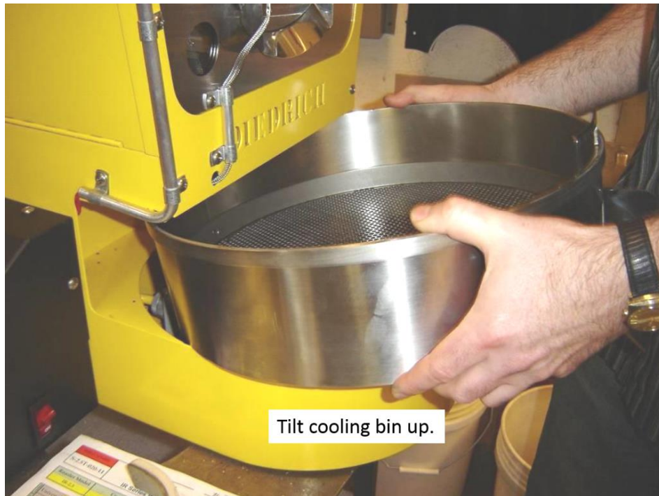
2.6.1.5 Tilt the front edge of the cooling bin up.
