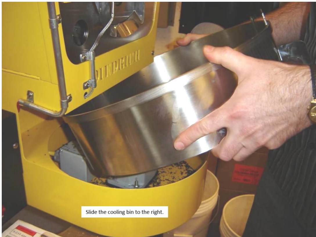
2.6.1.6 Slide the cooling bin to the right.
