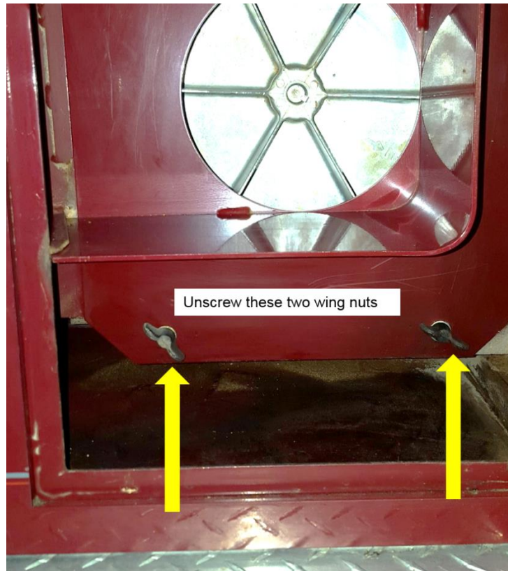
2.3.1 Unscrew the two wingnuts securing the impeller cover
